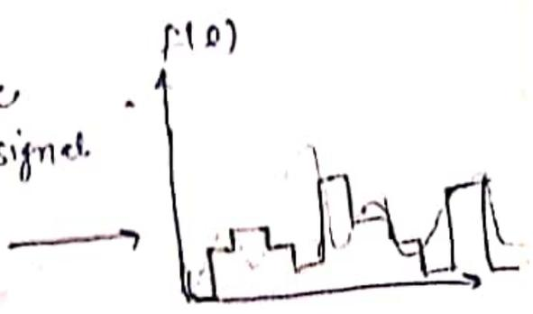
A digital to analog converter converts digital input signal into an analog output signal. The digital signal is represented with a binary code which is 0 and 1. In general, the number of binary input will be a power of two.
