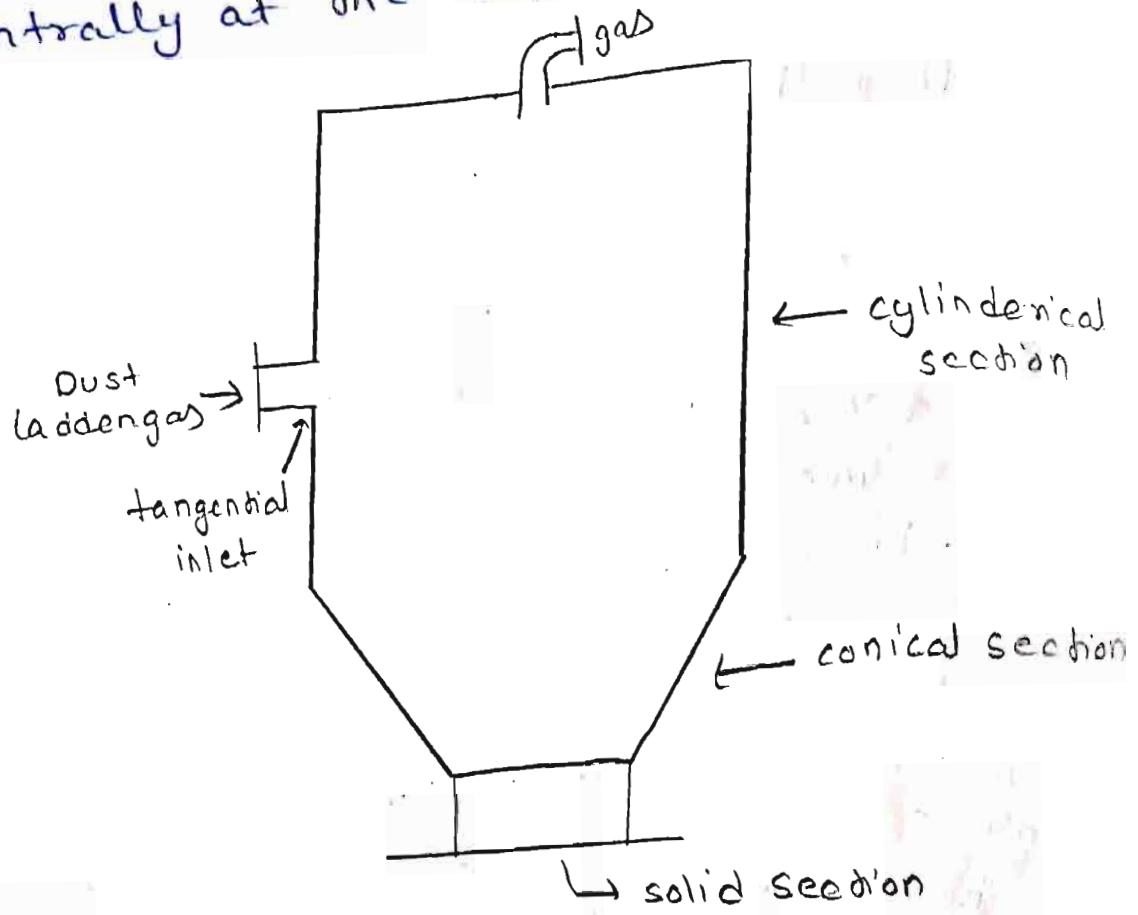
Working  $\Rightarrow$  The outlet is provided with a downward extending pipe. A pipe that extends upward into the cylindrical section to prevent the gas short circuiting directly from the inlet in the outlet and for cutting the vortex. In this separation used for the separation of due particles are most from ground. If dust loaded gas is introduced tangentially then a cylinder in vessel at a high velocity ( $30 \text{ m/s}$ ). Centrifugal force throws the solid particles out against the
