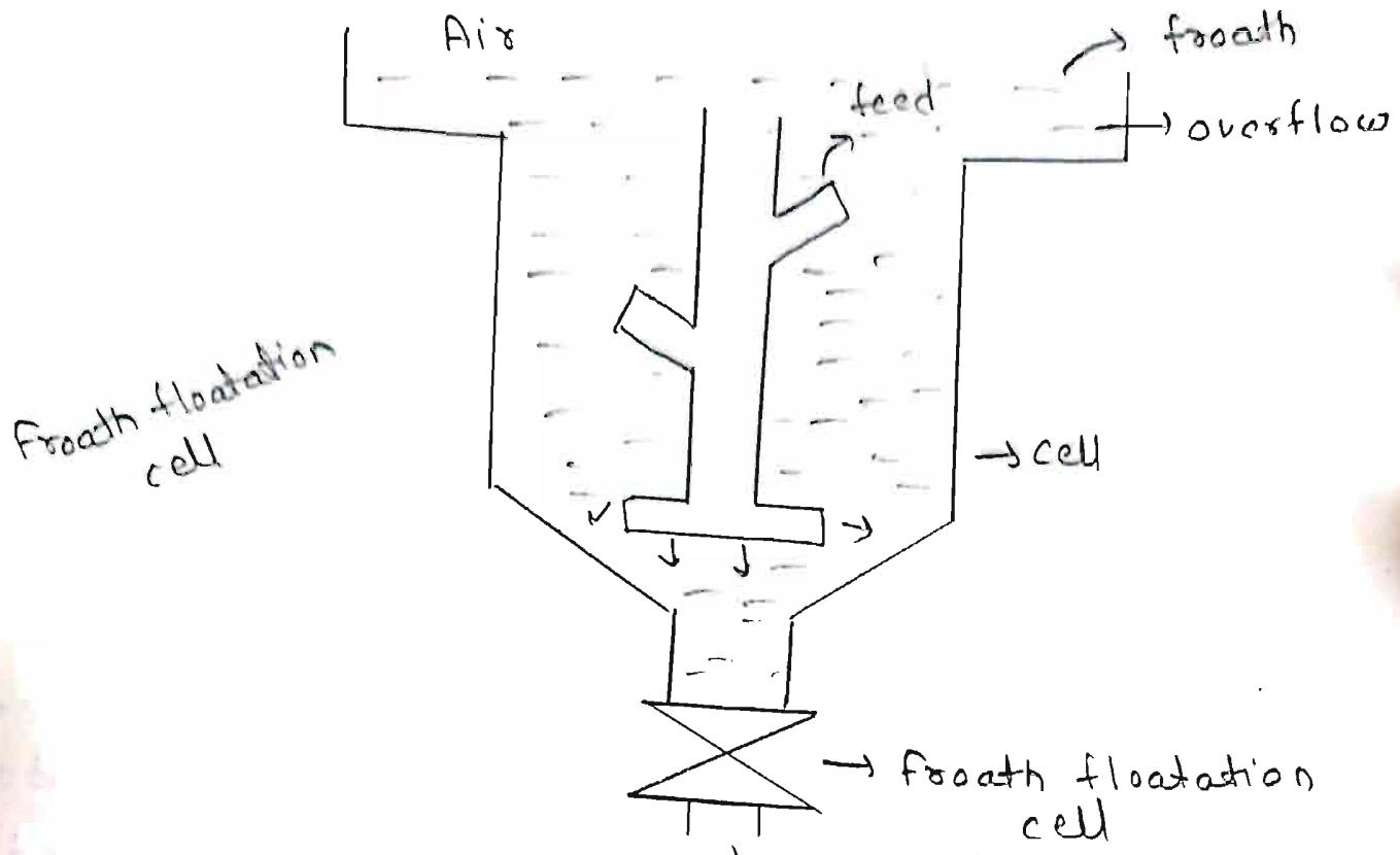
Working  $\Rightarrow$  Water is taken into the cell, material is feed to the cell. The promoters and froth are added. Agitators are given and air is bubbled into the form of fine bubbles. Air avid particles they are discharged from the overflow. Hydrophilic particles sink to the bottom and removed from the discharge for tailings.
