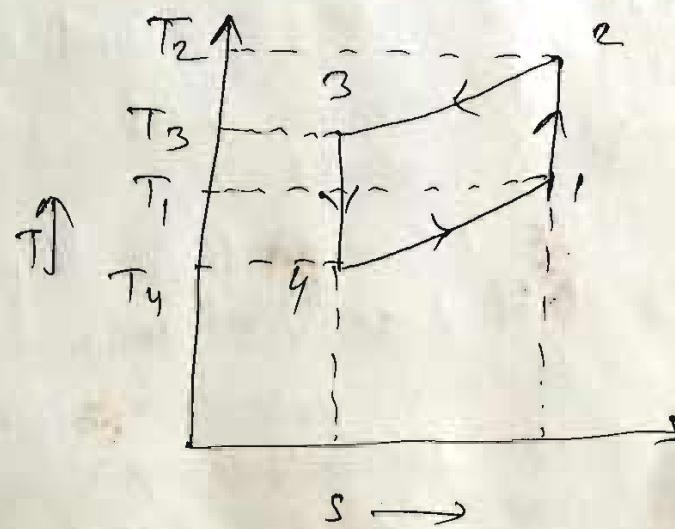
Process-(1-2)-Isentropic Compression— In this process air is drawn from evaporator (refrigerator) to compressor cylinder where it is compressed isentropically. No heat interaction takes place in this process. As the air is compressed, the volume decreases from  $V_1$  to  $V_2$ , pressure increases from  $P_1$  to  $P_2$  and Temp $^\circ$  increase to  $T_1$  to  $T_2$  but entropy remains constant.
