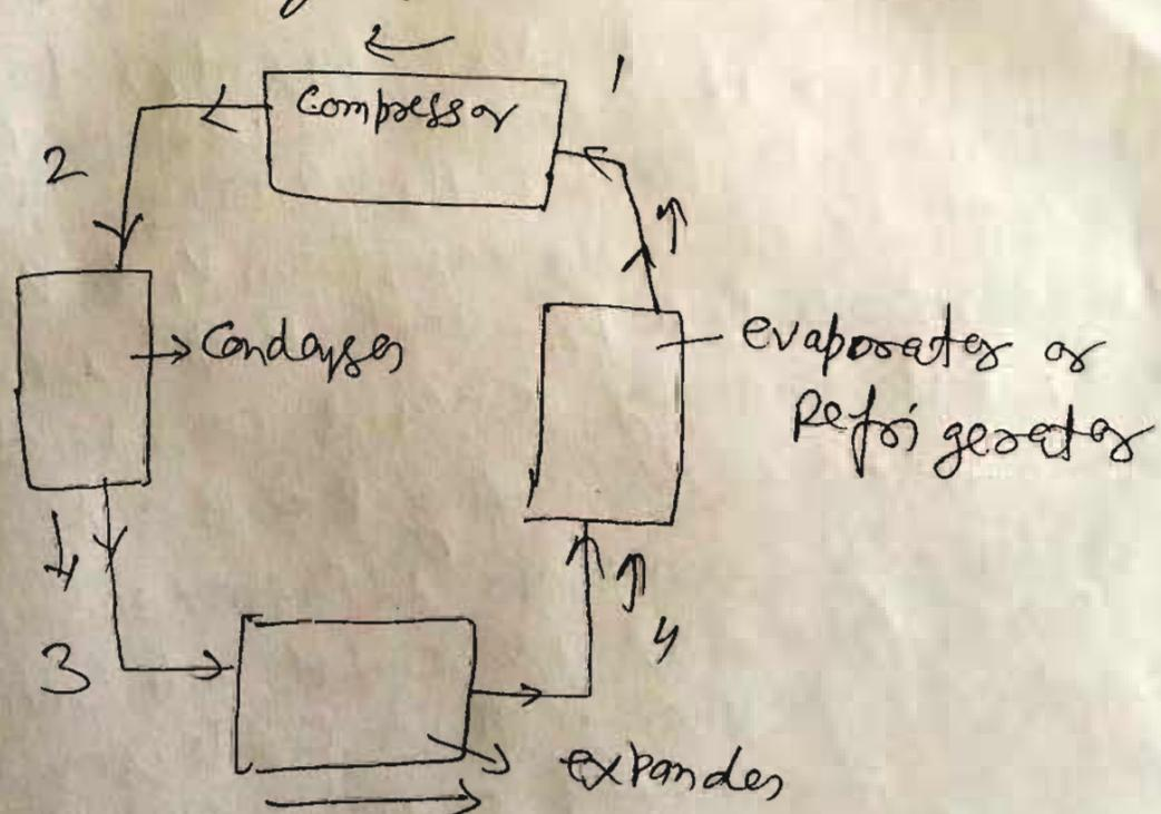
The above fig. shows the different processes in a Bell-Coleman cycle. This cycle consists of a compressor, a cooler or condenser, an expander & throttling device and a evaporator or refrigerator.
