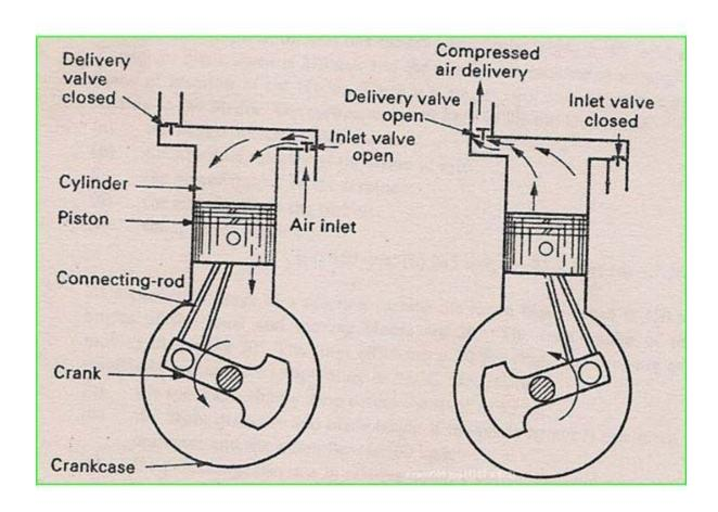
Reciprocating Air Compressor has also classified according to its stages. So, Classification will help you better understand the working of the reciprocating air compressor.
