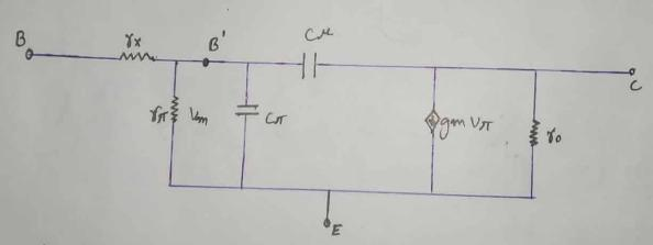
High fruequency Model Explained > In High foreignency model a gresistant and two Copaciator are added In addition to the Components in low foreignency Model.
