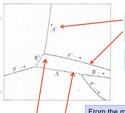
From the curvature radius we get the momentum of the charged particles and, by knowing the kind of particles, their energies.
